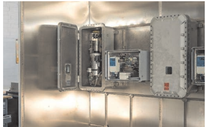
Figure 5: CWD2000 Ex for potentially explosive areas
